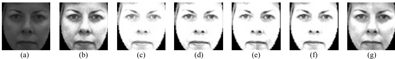
Fig. 3. Image examples: (a) Geometrically normalized and masked image with no enhancements (NE), (b) histogram equalized (HE), (c) homomorphically filtered image (HM), (d) homomorphically filtered and contrast adjusted image (HMADJ), (e) two vertical sub-images filtered separately (HMV), (f) two horizontal sub-images filtered separately (HMH), (g) proposed combination (HMMOD)
